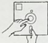
Do not write anywhere on the disk except on the label. Always write with a felt tip pen; do not use a pencil or ink pen.
