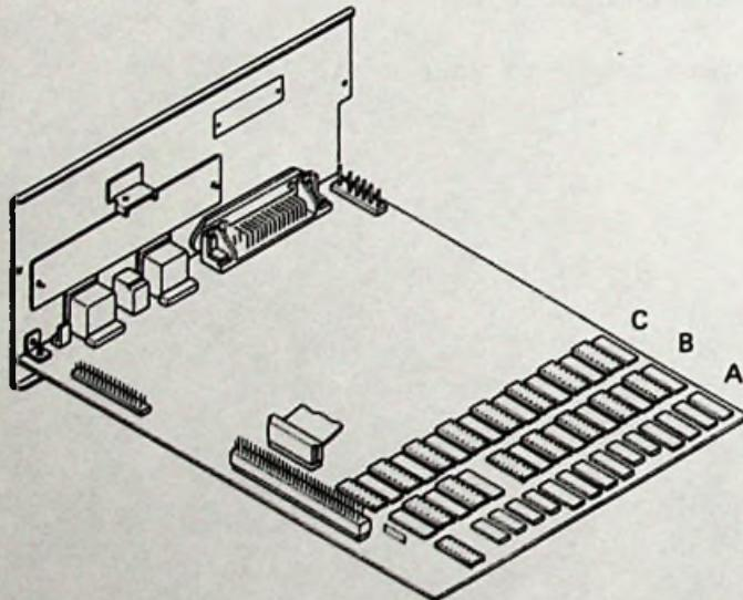
6) Seven memory chips will fit into the sockets in column B. One memory chip must be place in the last socket in column A. The order that you place the chips does not matter. How you insert the chips does. Look at a chip. One end is flat, one end has a half circle cut in it. This half circle should be facing toward the panel. All lettering on these chips and the ones in column B and A should be reading in the same direction.
