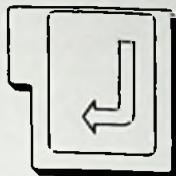
The RETURN key, indicated by a down left arrow, checks for valid commands and returns the cursor to home position. It starts new lines in basic mode.
