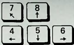
These "arrow" keys move the cursor one line or character per stroke and are accessed through software. The cursor keys are located on the ten key pad: key seven - cursor diagonally, key eight - cursor up, key four - cursor left, key five - cursor down, and key six - cursor right.
