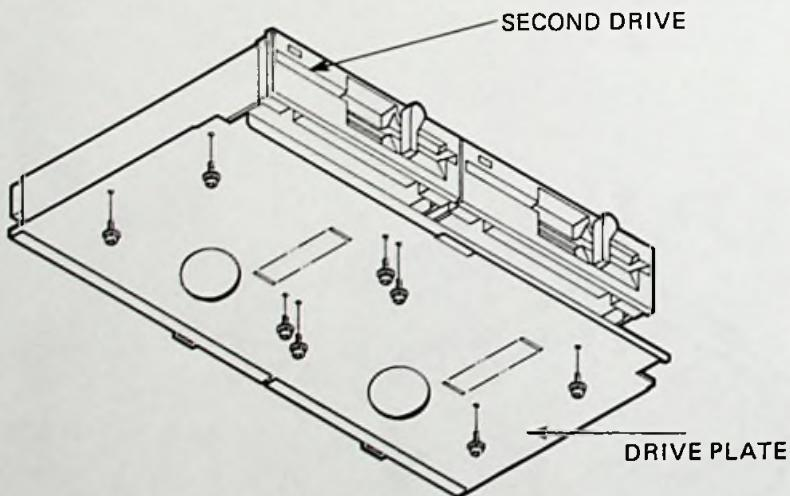
7) Replace the drive plate and the two drives back into the cabinet.
