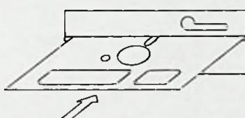
Hold the diskette by the label and insert into the drive. The write protect cut out on the disk edge will face left and the read/write slot will lead into the drive.
